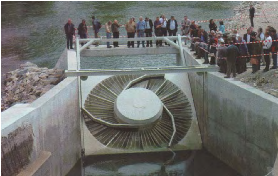
Abb. 8-6: Very-Low-Head Turbine, MJ2 Technologies SARL, Quelle: WP&Dams, 5, 2008
